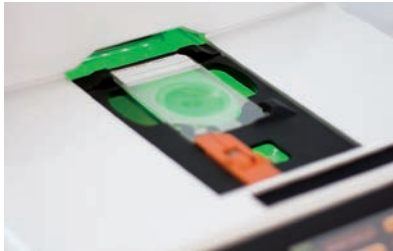
6. Green light signals completion of heat stabilization.
