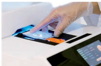
4. Place sealed Maintainior® tissue card into Stabilizor™ system.
