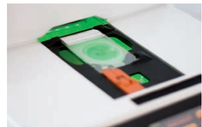
6. Green light signals completion of heat stabilization.
