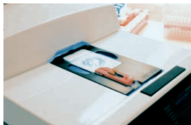
5. Air is evacuated and sample enters instrument.
