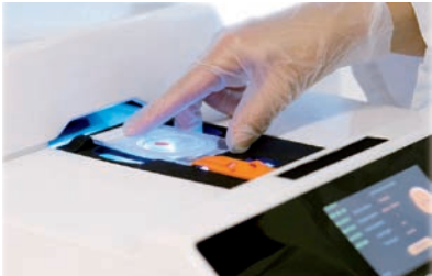
4. Place sealed Maintainer® tissue card into Stabilizor™ system.
