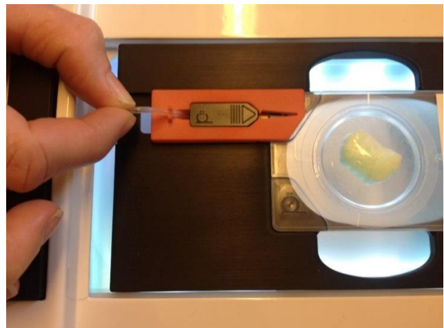
Figur 1. The clear plastic tube connecting the cavity, through the needle, with the vacuum system is pinched to stop the cavity from being evacuated and prevent morphological deformation by the upper foil.
