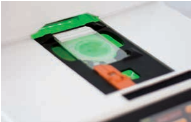
6. Green light signals completion of heat stabilization.
