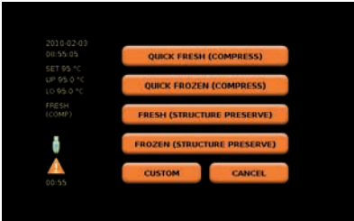
1. Select program for fresh or frozen samples, input sample details.
